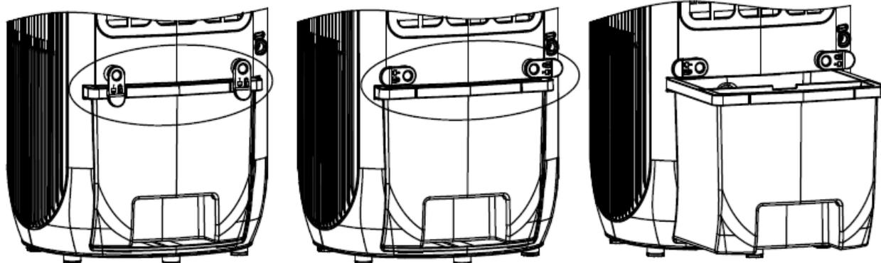
3. Fill the water tank with a watering can, take into account the maximum water level indicator, see at the front of the device.
